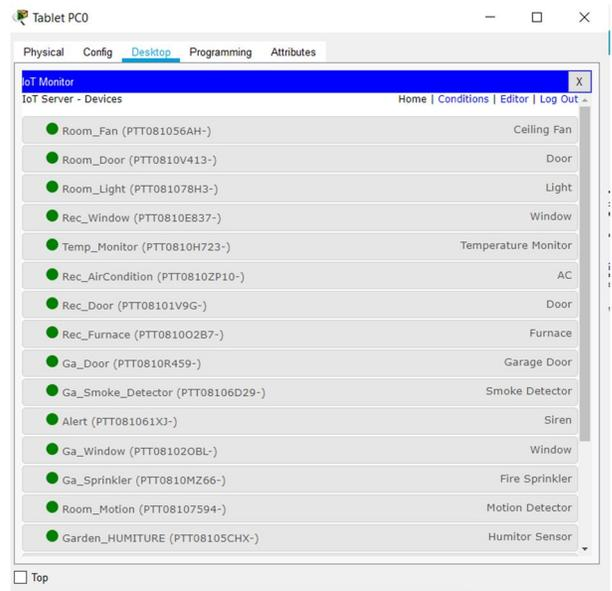
FIGURE 3: A list of the network-connected devices that are connected to the IoT Server.
